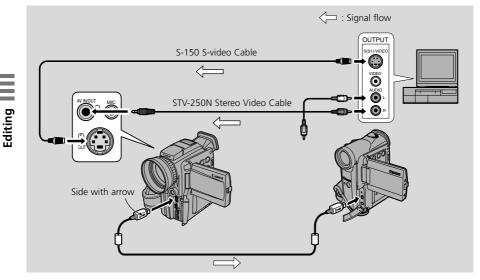
Above illustration shows the connection using a S-video cable. You can also connect to the VIDEO terminal instead ( $\square$  38).
